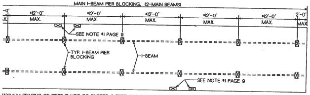
IAXIMUM SPACING OF PIERS IS NOT TO EXCEED 8 FEET FOR 8 INCH I-BEAM, 10 FEET FOR 10 INCH I-BEAM AND FEET FOR 12 INCH I-BEAM.
