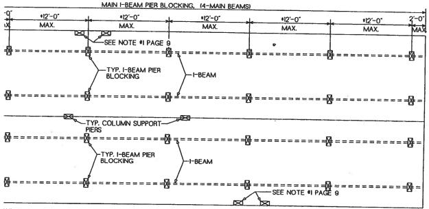
\XIMUM SPACING OF PIERS IS NOT TO EXCEED 8 FEET FOR 8 INCH I-BEAM, 10 FEET FOR 10 INCH I-BEAM AND FEET FOR 12 INCH I-BEAM.
