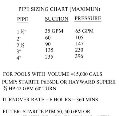
TURNOVER RATE = 6 HOURS = 360 MINS. FILTER: STARITE PTM 50, 50 GPM OR HAYWARD C751, 75 GPM CAPACITY MAIN DRAIN: HAYWARD W61048E CLEANER: HAYWARD VAC LOC
