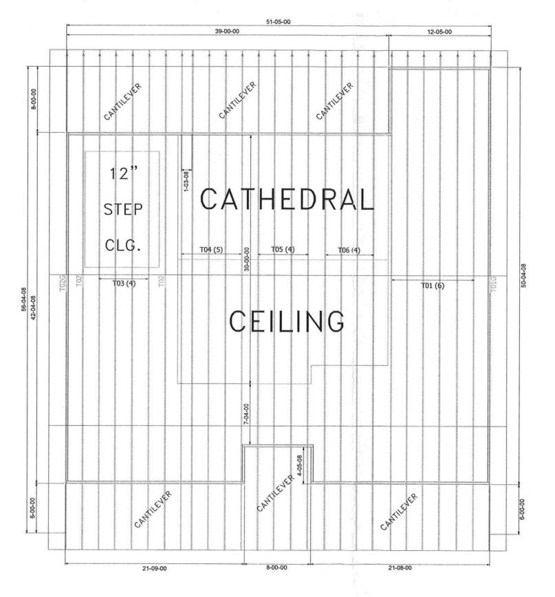
THE ARROW HEAD AT THE END OF THE TRUSS ON THE TRUSS PLACEMENT CORRESPONDS WITH THE LEFT SIDE OF THE INDIVIDUAL TRUSS DRAWING, USE THIS AS AN DRIENTATION GUIDE WHEN SETTING THE STRUCTURE.
