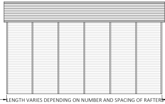
TYPICAL SIDE ELEVATION - HORIZONTAL ROOF
