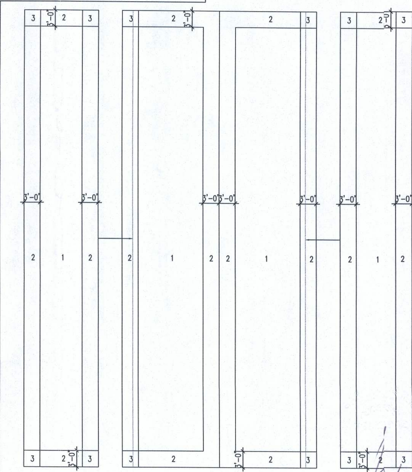
ROOF FASTENING PLAN 3/32" = 1'
