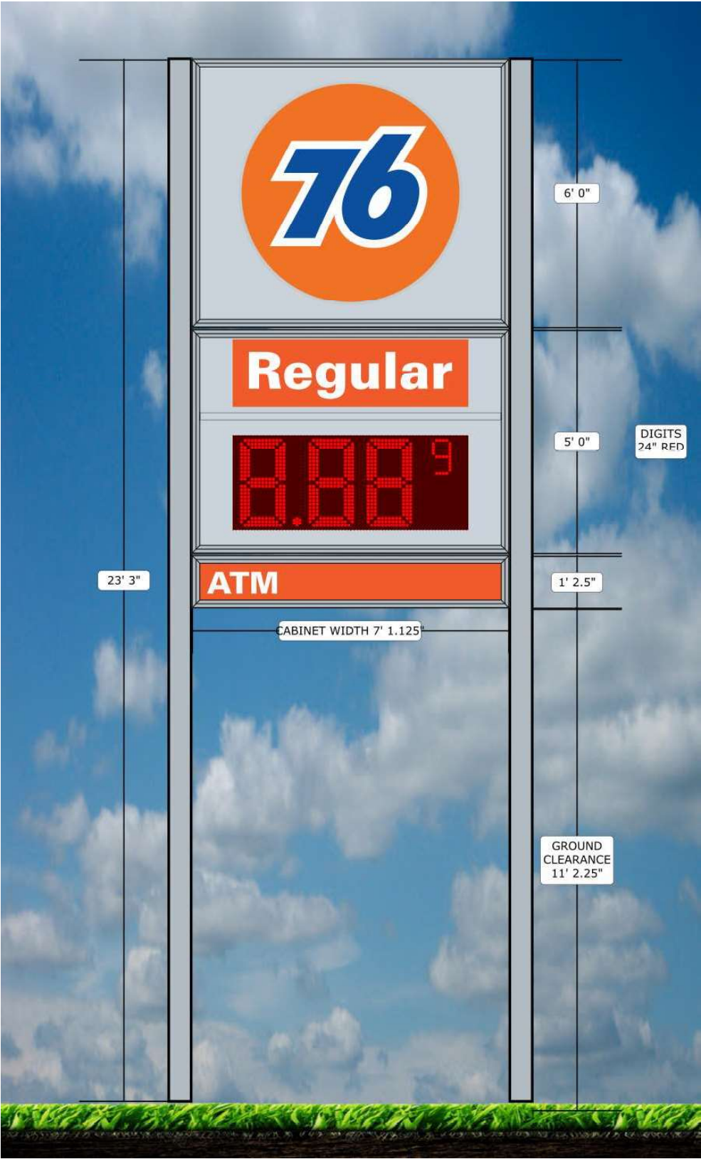
ELEVATION DRAWING OF NEW SIGN STRUCTURE
