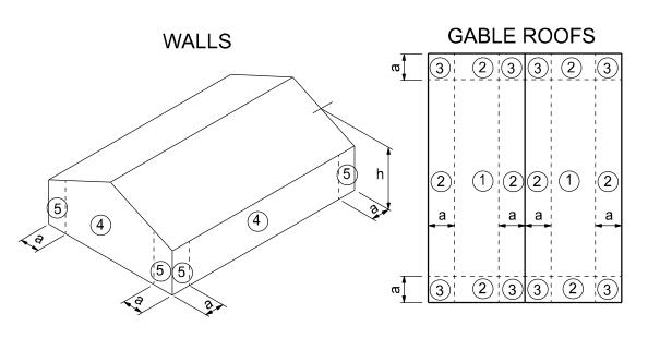
a: 10% of least horizontal dim. or 0.4h, whichever is smaller, but not less than either 4% of least horizontal dimension or 3 ft.
