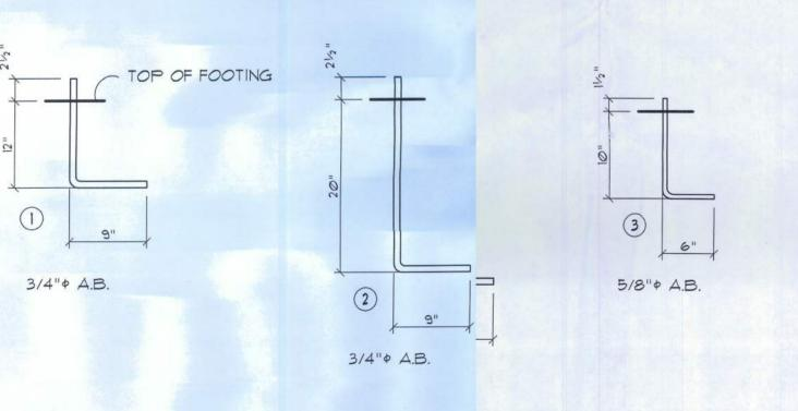
NOTE! ALL ANCHOR STEEL ROD, OR BOLTS ARE ASTM GRADE A36 BLACK, AND D. THREADED 3", OR GRADE A301, ID FREE FROM RUST AND SCALE
