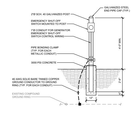
**EMERGENCY SHUT-OFF SWITCH DETAIL**
