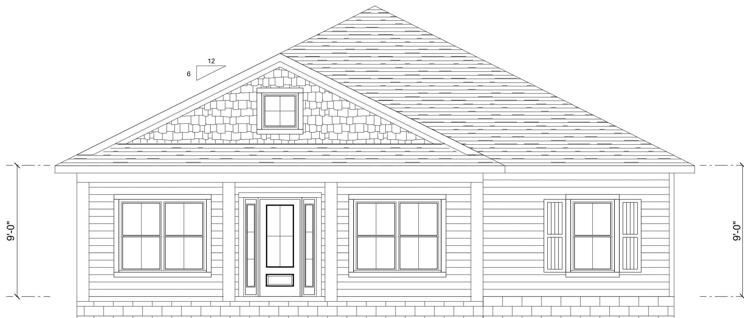
FRONT ELEVATION SCALE: 1/4" = 1'-0"
