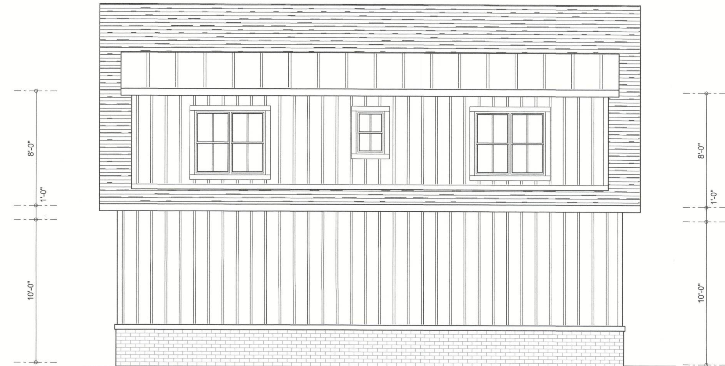
REAR ELEVATION SCALE: 1/4" = 1'-0"
