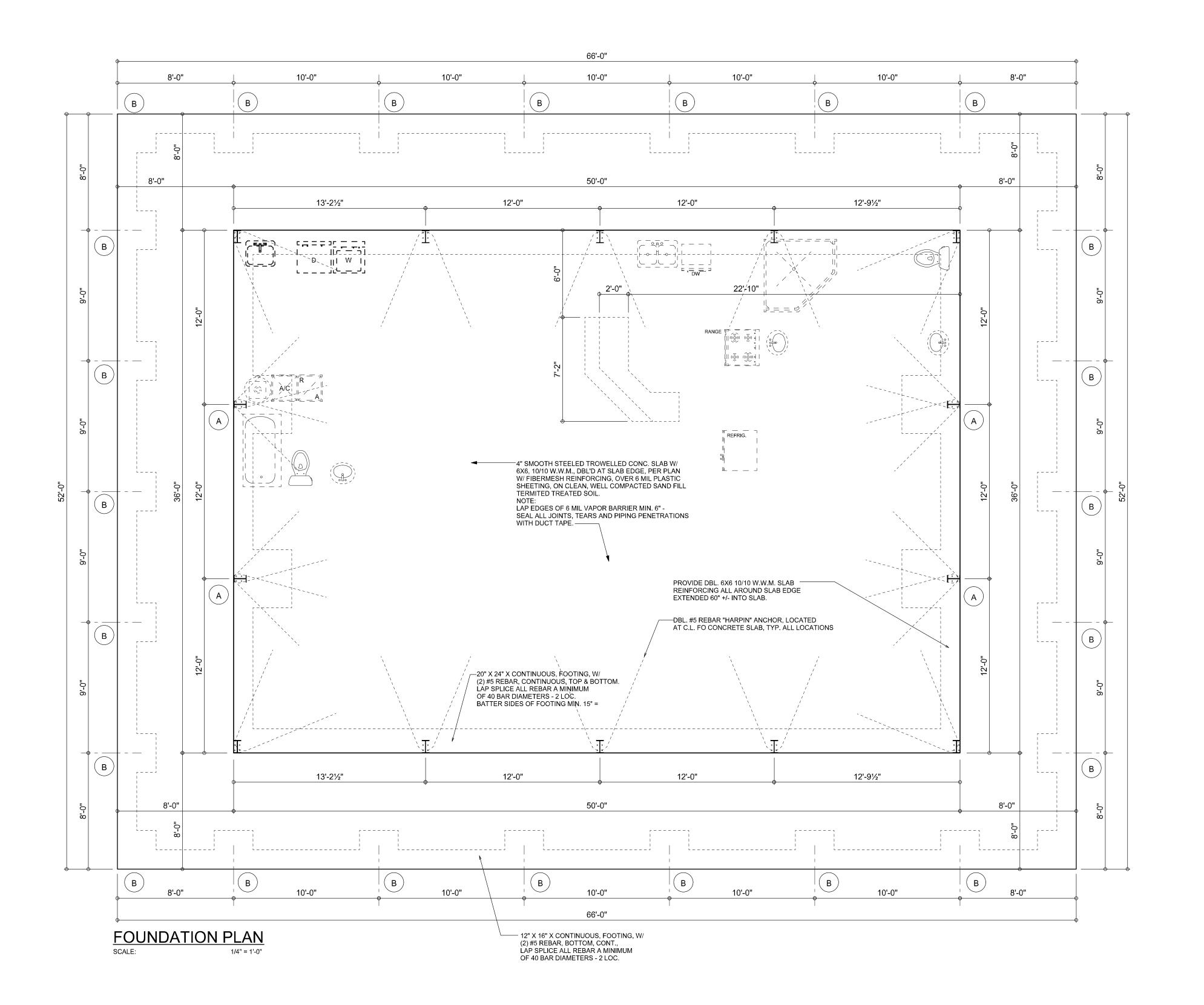
NOTE: THIS FOUNDATION DESIGN MEETS ALL REQUIREMENTS FOR WIND LOAD'S PER PROJECT IS 130 MPH PER 2017 PER R301.2.1.1 BASIC WIND SPEED, EXPOSURE B, 1.0 USE FACTOR. COLUMN PAD LOCATIONS ARE TYPICAL, EXACT ANCHOR BOLT LOCATIONS AND SIZES ARE PER METAL BUILDING SEALED ENGINEERING ANCHOR BOLT PLAN. CONTRACTOR SHALL FURNISH ARCHITECT SEALED METAL BUILDING PLANS FOR FOUNDATION SIZING AND VERIFICATION PRIOR TO SUBMITTING TO PERMIT OFFICE.
