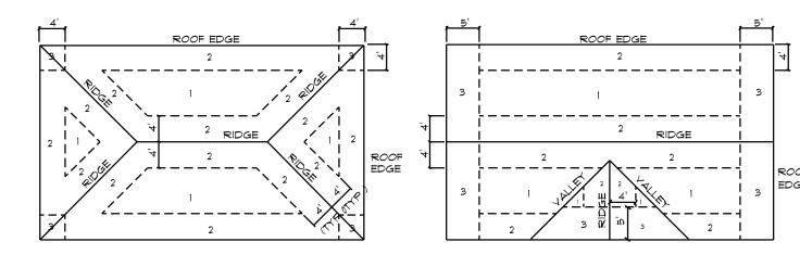
ROOF SHEATHING NAILING ZONES (HIP ROOF)
