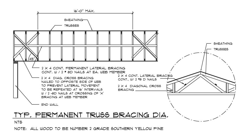
Truss Bracing DETAILS
