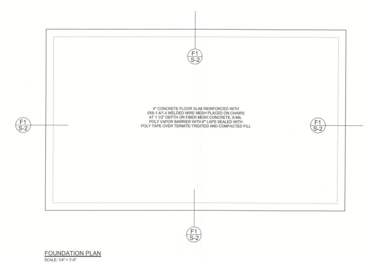
DIMENSIONS ON STRUCTURAL SHEETS ARE NOT EXACT. REFER TO ARCHITECTURAL FLOOR PLAN FOR ACTUAL DIMENSIONS
