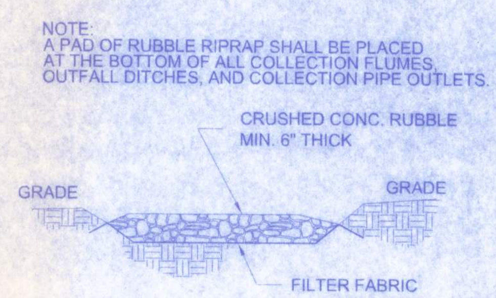
RUBBLE PAD DETAIL NTS
