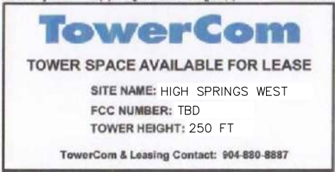
OWNER CONTACT SIGN WHITE BACKGROUND, BLACK/BLUE LETTERING. 20"x24" ALUMINUM SIGN WITH 1/4" DRILLED HOLES IN EACH CORNER THICKNESS: 0.05" (1/16") OR CLOSEST STANDARD THICKNESS MOUNTING LOCATION: GATE AND ACCESS ROAD GATE IF APPLICABLE QUANTITY: 1 (IF 2) HANG ON OUTER GATE(S))
