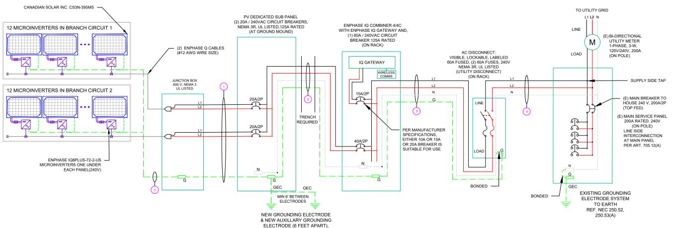
REQ. 5/8" DIA GROUNDING ROD WITH 8' MIN. EMBEDMENT
