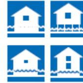
For example, this series of figures from the guide shows how a house on a basement or crawlspace foundation can be elevated above the flood level on extended foundation walls.
