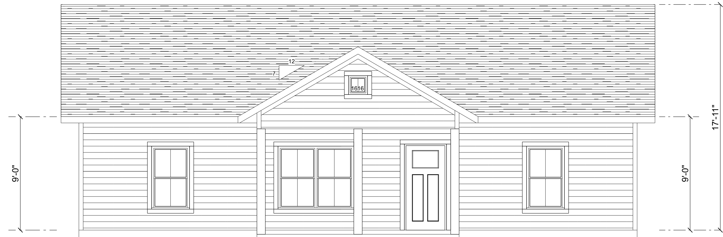
FRONT ELEVATION SCALE: 1/4" = 1'-0"
