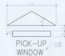
PAVEMENT MARKER DETAIL
