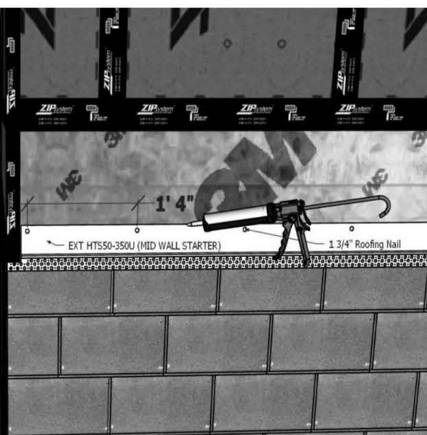
3 MID-WALL STARTER STRIP: ANGLE SET 1" BELOW TOP OF CMU. ATTACH w/ 1 3/4" ROOFING NAIL @ 16" O.C. RUN SMALL BEAD OF CAULK @ THE TOP OF JOINT & FLASHING MEMBRANE AS ADDED PROTECTION
