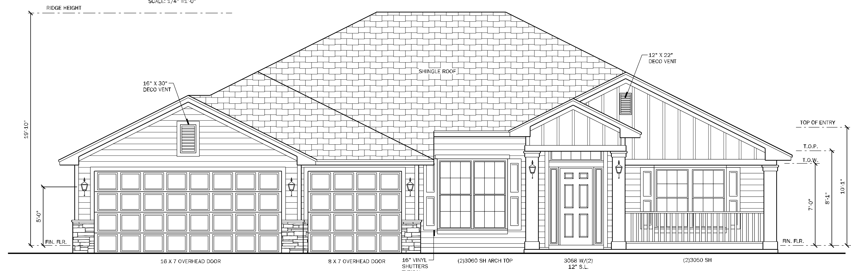
FRONT ELEVATION "C" SCALE: 1/4" = 1'-0"
