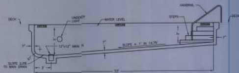
POOL SECTION SCALE: 1/4"=1'-0"
