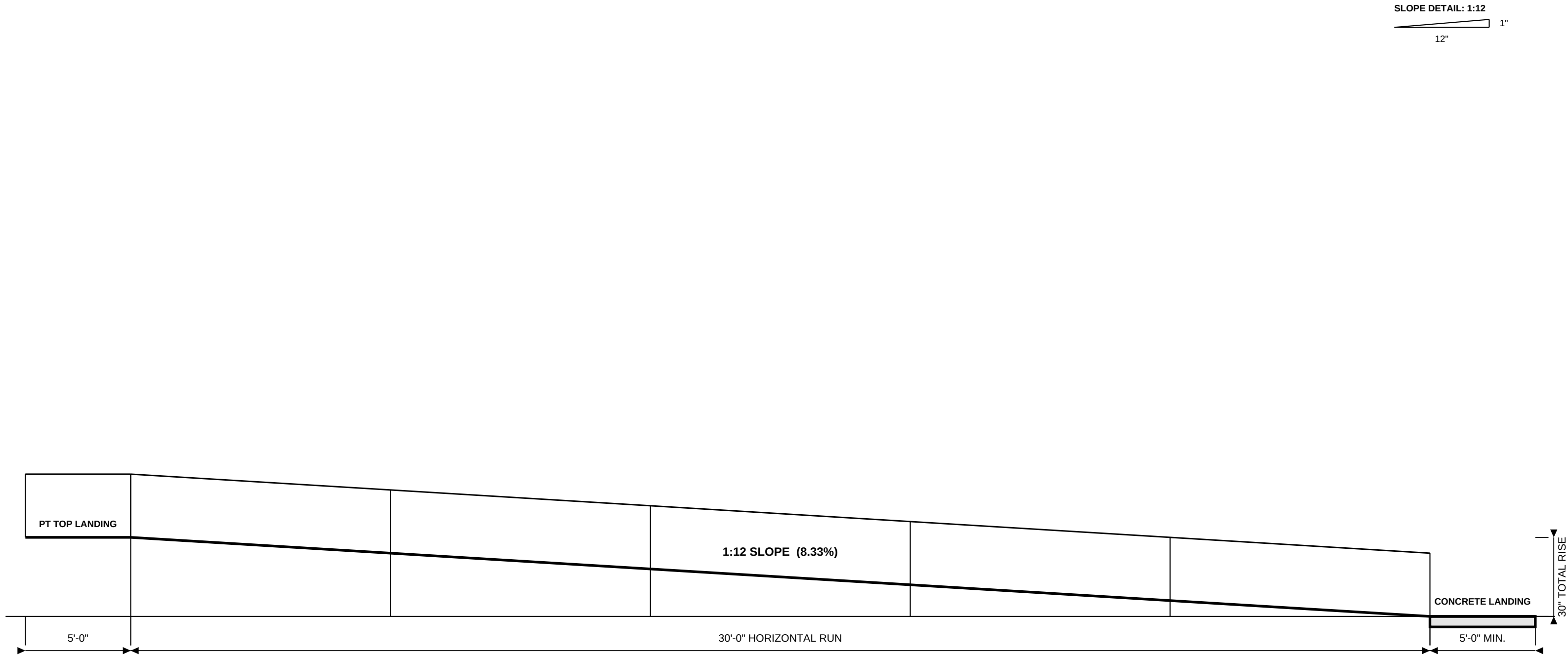
FRONT RAMP - SIDE ELEVATION
