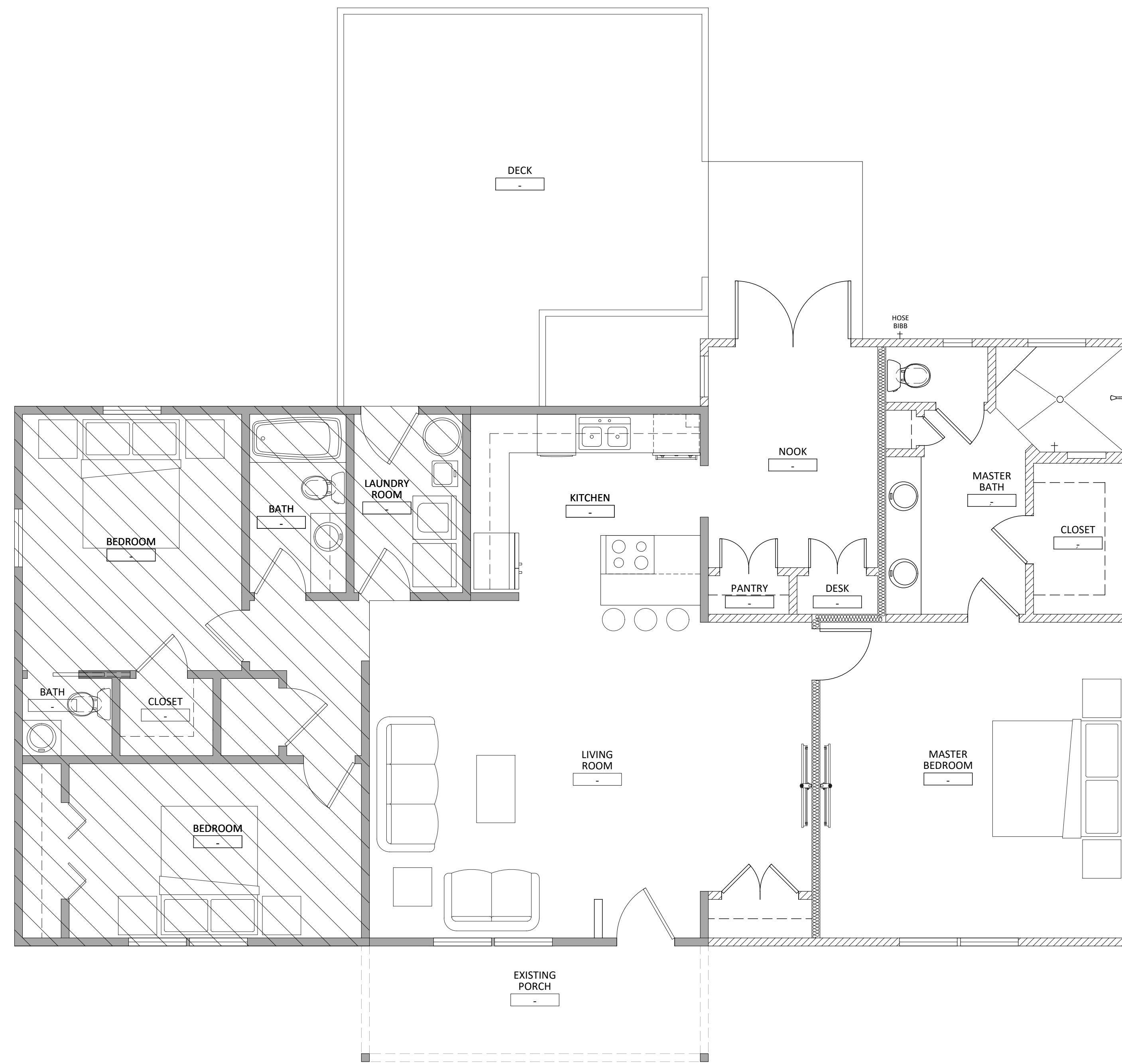
1 Overall Floor Plan (Shown without tags or dimensions to show completed design intent) Scale: 1/4" = 1'-0"
