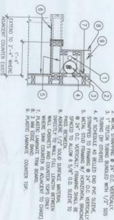
15 DIALYSIS COUNTER END WALL / VERTICAL CHASE SCALE 3/4" = 1'-0" (A7-28 R10)
