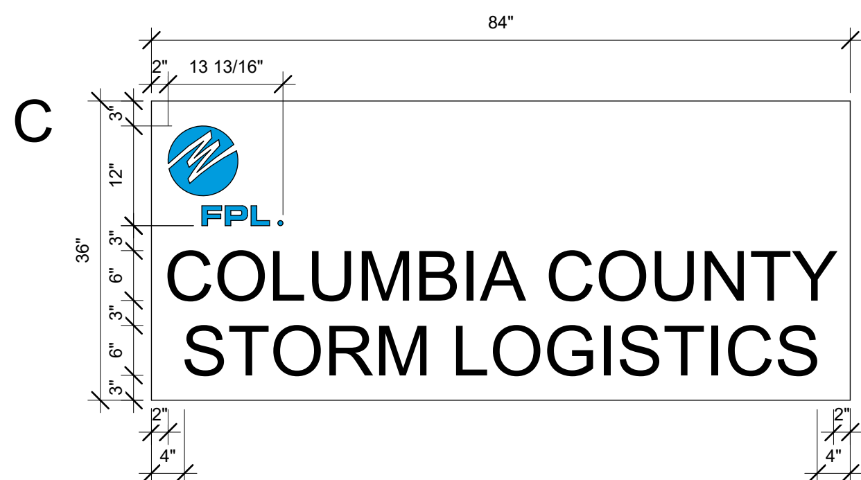
3 BUILDING SIGNAGE TYPE 2X - BUILDING DESIGNATION B-A601 3/4" = 1'-0"
