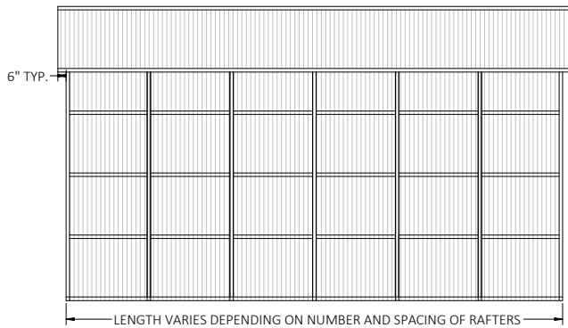
TYPICAL SIDE ELEVATION - VERTICAL ROOF/SIDING OPTION
