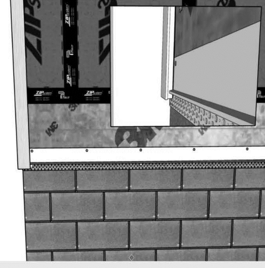
4 TRIM: CORNER TRIM SET INTO NOTCH MIN. 3/4" BELOW TOP OF CMU. INSTALL PER MANUFACTURER INSTRUCTIONS.
