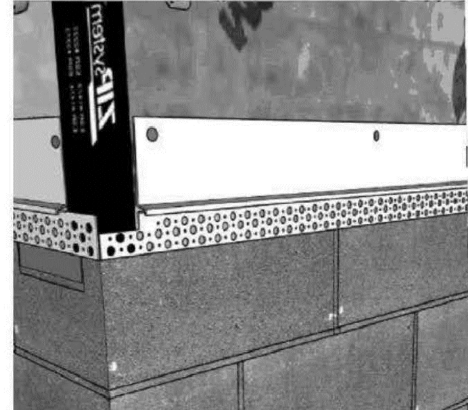
MID-WALL STARTER STRIP: NOTCH CORNER TO ACCEPT TRIM BEFORE INSTALLING. NOTCH TO EXTEND MIN. 3/4" BELOW TOP OF CMU
