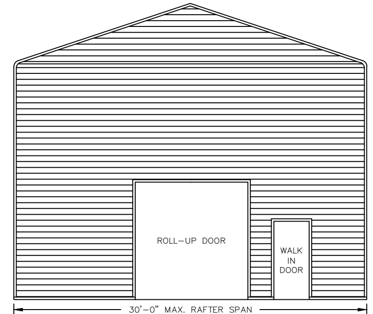
TYPICAL ELEVATION - BOW EAVE SCALE: NTS
