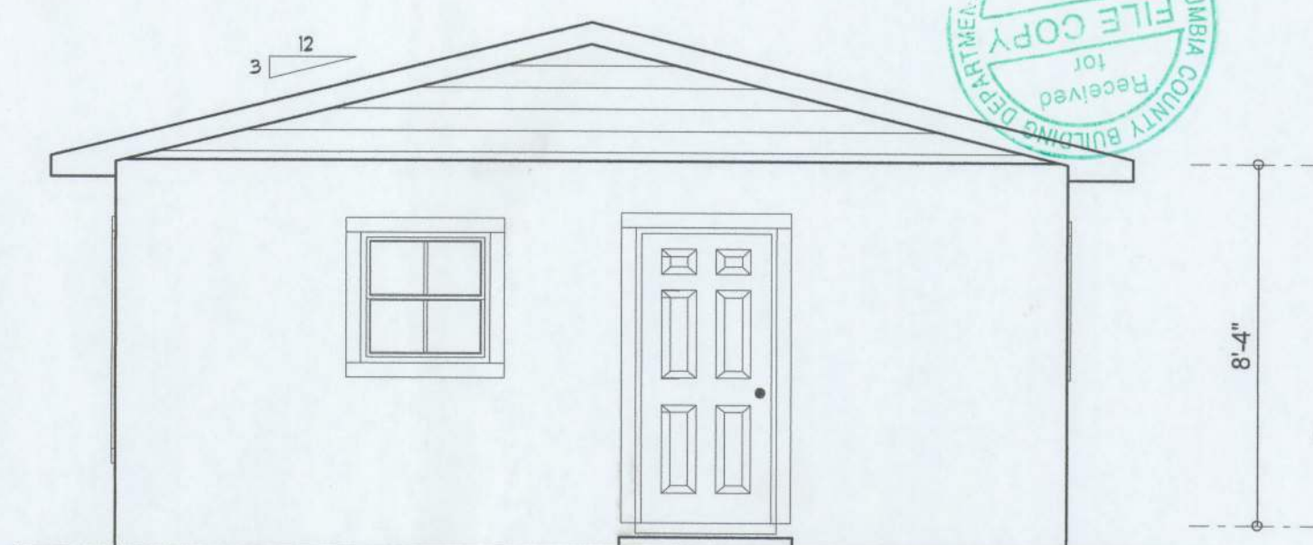
FRONT ELEVATION SCALE: 1/4" = 1'-0"
