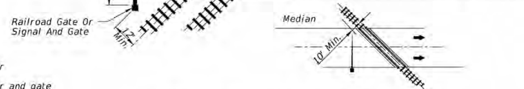
SIGNAL PLACEMENT AT RAILROAD CROSSING (4 - LANE DESIGN)
