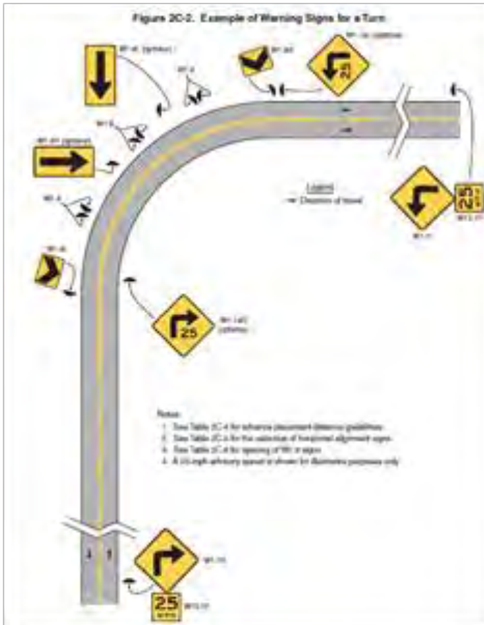
Figure 20. Signs for curve (modify curve/turn signs to reflect minor intersecting streets)
